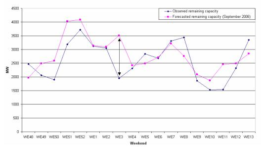
Figure 2 Forecasted Remaining Capacity Verses Observed Remaining Capacity (Weekends)
