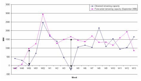
Figure 2 gives an overview of the forecasted remaining capacity (evaluation time September 2006) and the observed remaining capacity for the weekend peaks of the winter 2006-2007.
