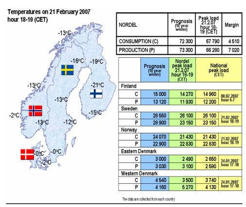
EXCHANGE AT PEAK LOAD ON 21 FEBRUARY 2007 (18-19 HOURS, CET) [MWh/h]
