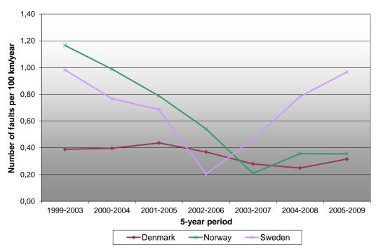
Figure 5.7 Fault trend for cables at all voltage level.
