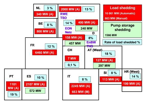
Figure 7: Map of load and pumped-storage shedding by TSOs
