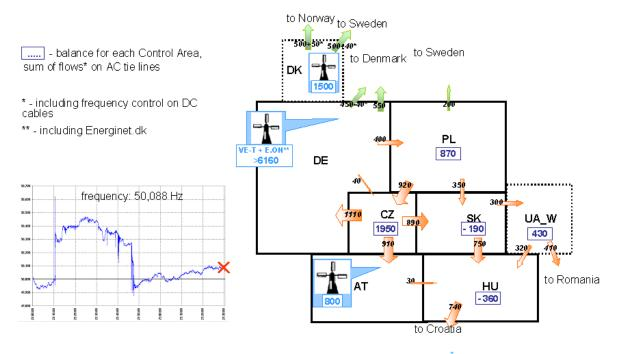
Figure 22: Intersystem power flows in area 2 at 23:30 (back to normal operational conditions)
