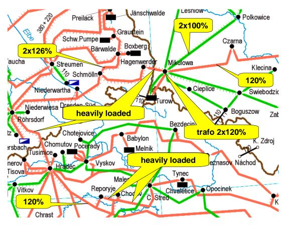
Figure 18: Overloaded elements in the region of VE-T/PSE-O/CEPS borders
