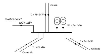
Figure 30: Landesbergen substation - After coupling both busbars
