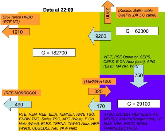
Figure 1: Generation and power flows between the 3 areas just before splitting 4 November 22:09
