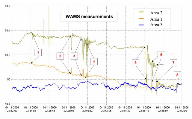
Figure 25: Frequency recordings for three areas
