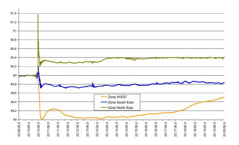
Figure 6: Frequency recordings after the split
