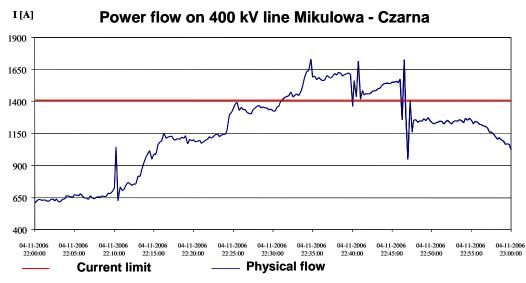
Figure 20: Overloads on the 400 kV Mikulowa-Czarna internal PSE-O line
