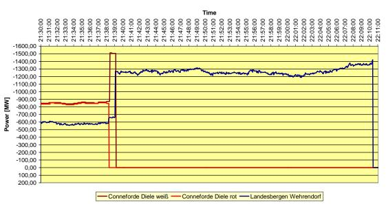
Figure 3: Power flow on the Landesbergen-Wehrendorf line before and after Conneforde-Diele switching off
