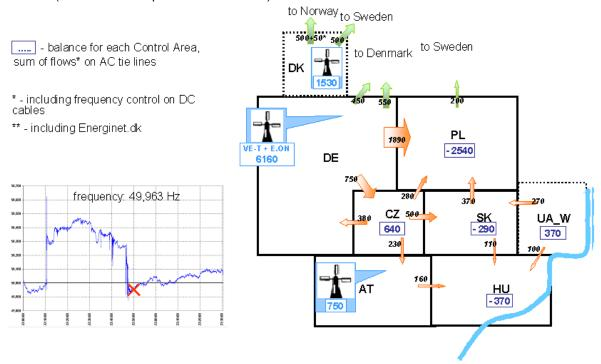
Figure 21: Intersystem power flows in area 2 at 22:50 (critical W-E flow just after synchronization in DE and A; decrease of W-E flow)
