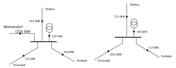
Figure 29: Landesbergen substation - Before coupling
