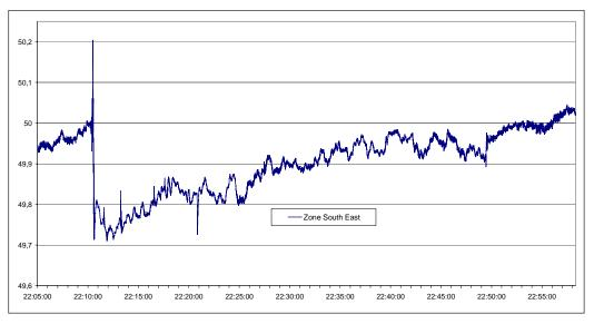
Figure 23: Frequency evolution in area 3 during the event (WAMS recording)
