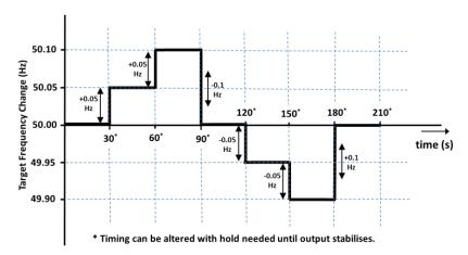
ECP.A.5.8 Figure 3 – **Target Frequency** setting changes
