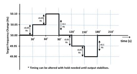
OC5.A.3.6. Figure 3 - Target Frequency setting changes
