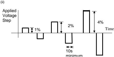
OC5.A.3.5 Figure 2 – Step injection sequence for voltage control tests
