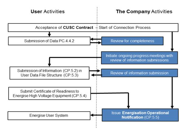
The process illustrated in CP.A.1.1 applies to all **GB Code Users** energising passive network **Plant** and **Apparatus** including **Distribution Network Operators**, **Non-Embedded Customers**, **Generators** and **DC Converter Station** owners. This process is a subset of the full process for **Generators** and **DC Converter Station** owners shown in CP.A.1.2. This diagram illustrates the process in the **CP** and includes references in brackets to specific Grid Code clauses.
