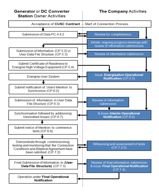
This diagram illustrates the process in the **CP** and includes references in brackets to specific Grid Code clauses. For the avoidance of doubt this process does not apply to **Embedded Medium Power Stations** not subject to a **Bilateral Agreement** and **Embedded DC Converter Stations** not subject to a **Bilateral Agreement**.
