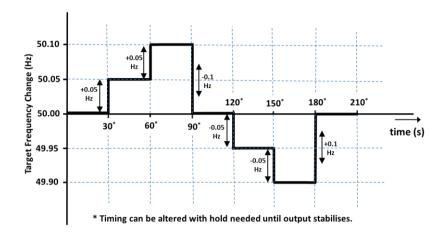
OC5.A.4.6. Figure 3 – Target Frequency setting changes
