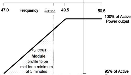
Note: **Frequency** F<sub>LFDD-1</sub> is the relay trip setting of the first stage Power output of the Automatic Low **Frequency Demand Disconnection**Scheme
