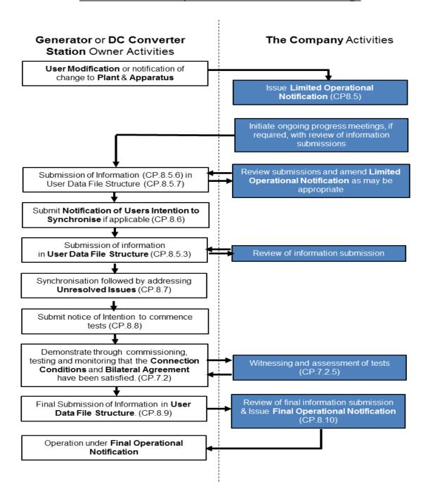
This diagram illustrates the process in the **CP** and includes references in brackets to specific Grid Code clauses. For the avoidance of doubt this process does not apply to **Embedded Medium Power Stations** not subject to a **Bilateral Agreement** and **Embedded DC Converter Stations** not subject to a **Bilateral Agreement**.
