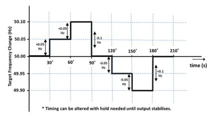
Figure 3 – Target Frequency setting changes
