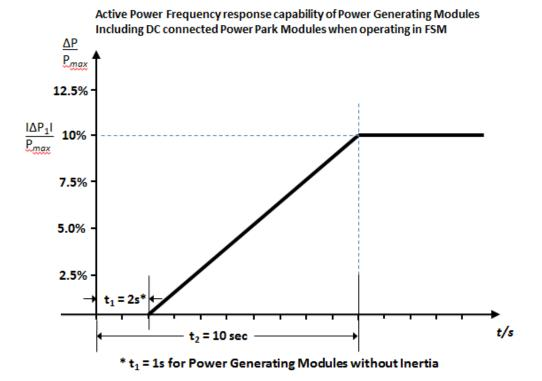
Figure 6.3.7.3.3(b) Active Power Frequency Response capability.
