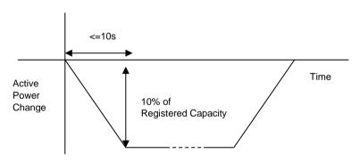
OC5.A.4.3 Figure 2 – Active Power ramp for reactive transfer tests
