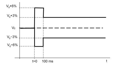
Figure CC.6.1.7 (1) — Voltage characteristic for frequent events
