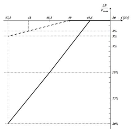
Figure 2D. Admissible limits for power reduction established by the TSO in case of underfrequency
