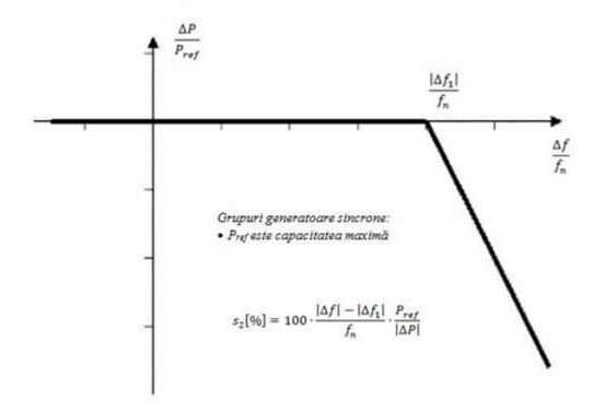
Figure 1C. Active power frequency response capability of type C synchronous power-generating modules in LFSM-O
