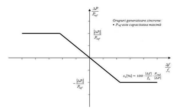
where:  $P_{ref}$  is the active power reference based on which the active power change  $\Delta P$  is established;  $\Delta P$  is the variation of the active power output from a synchronous power-generating module;  $f_n$  is the nominal frequency (50 Hz) in the network and  $\Delta f$  is the frequency deviation in the network.
