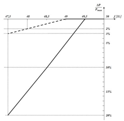
Figure 2B. Admissible limits for power reduction established by the TSO in case of underfrequency
