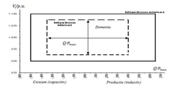
Figure 7D. U-Q/P<sub>max</sub>-profile of a synchronous power-generating module
