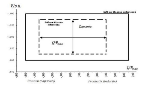
Figure 7C. U-Q/P<sub>max</sub>-profile of a synchronous power-generating module
