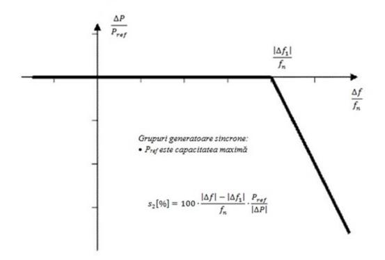
Figure 1A. Active power frequency response capability of type A synchronous power-generating modules in LFSM-O
