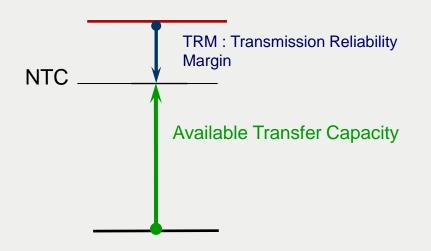
Allocation: based on the principle that an exchange from bidding zone A to bidding zone B uses the  $NTC_{A>B}$  defined on the respective Bidding Zone Border
