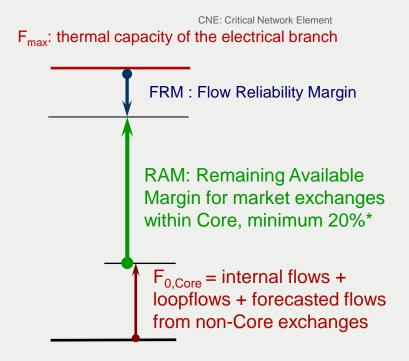
Allocation: optimizes exchanges by considering how much RAM each exchange uses on each CNEC (relationship = PTDF)
