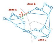
can be interconnectors or internal lines and can be monitored in a 'N situation' but also under outage scenario's 'N-1'. In the picture, the small 'b' is the CNE and the green 'a' the Contingency (C). The circles are nodes and the straight lines are the TSOs overhead lines.
