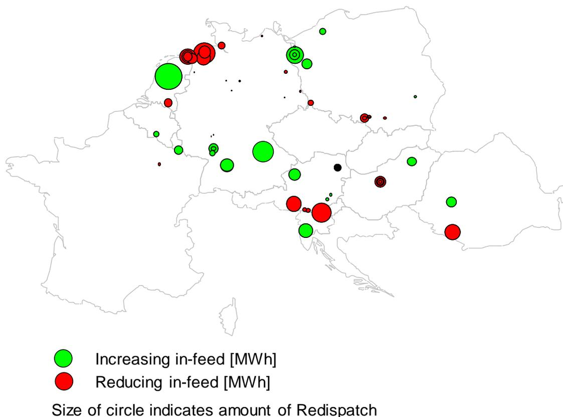
*Figure 4: Exemplary result of a Core-wide Redispatching optimization*
