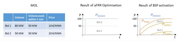
Figure 9: Example of MOL deviations due to dynamic constraints
