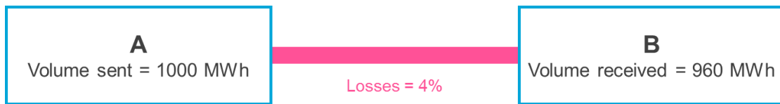
Figure 27: Example of Power Flow Losses on an HVDC Link
