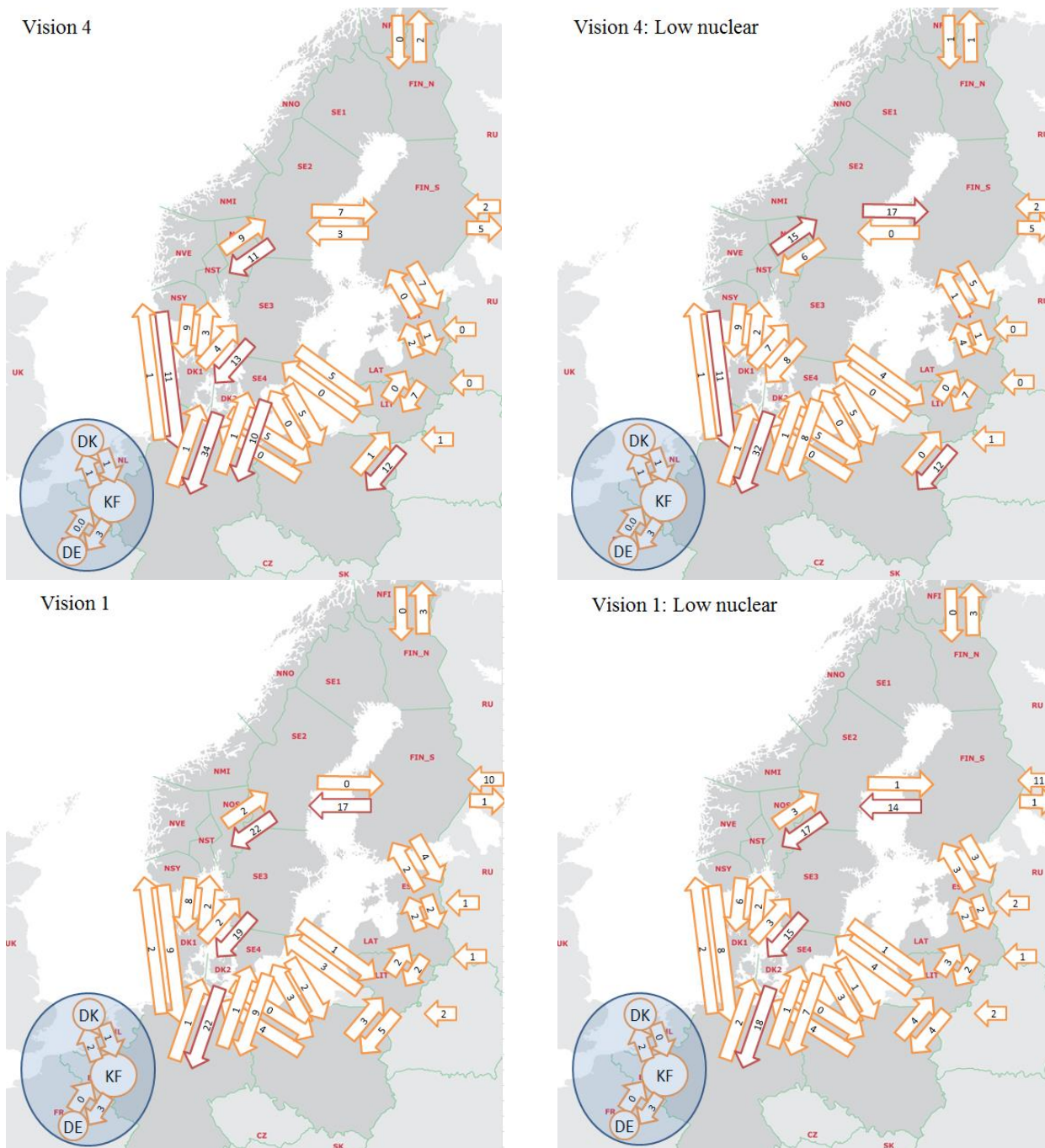
Figure 105 Energy flows in TWh; comparison of reference case with sensitivity case, Visions 1 and 4.
