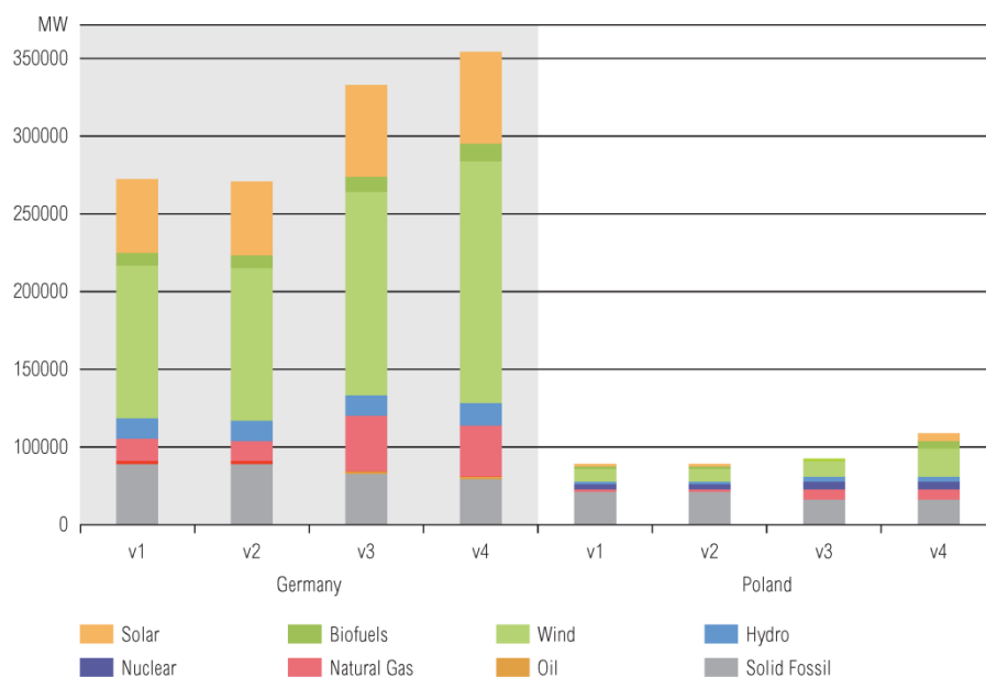
Figure 87 Generation portfolio mixture in Germany, Poland for each Visions 1, 2, 3 and 4, installed generation capacity in MW
