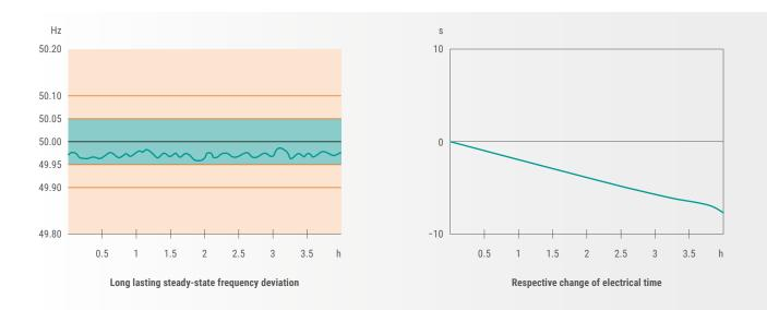
Figure 1: Relationship between frequency deviation and electrical time
