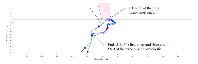
FIGURE 8-9: TRAJECTORY OF APPARENT IMPEDANCE MEASURED IN THE SLAVĚTICE SUBSTATION
