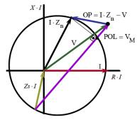
The mho characteristic operates when the angle between the operating quantity and the polarizing quantity is less than 90 degrees:
