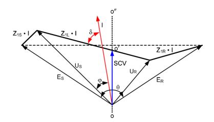
FIGURE 6-3 VOLTAGE PHASOR DIAGRAM OF A TWO-SOURCE SYSTEM
