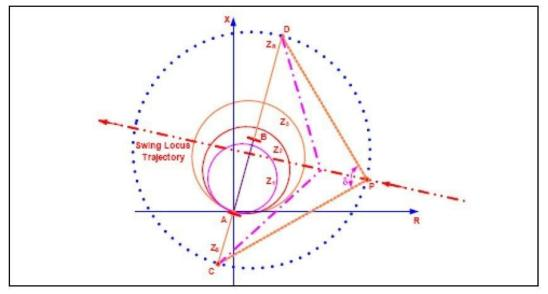
Figure 3-2: Swing locus trajectory when the magnitude of ES/ER = 1.0
