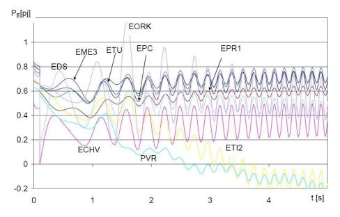
FIGURE 8-7: CALCULATED OUTPUTS OF POWER STATIONS CONNECTED INTO AFFECTED PART OF NETWORK
