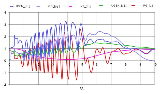
FIGURE 8-11: SIMULATION OF HYPOTHETIC LOSS OF STABILITY
