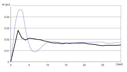
FIGURE 8-6: MEASURED AND SIMULATED TIME COURSE OF SPEED DEVIATION
