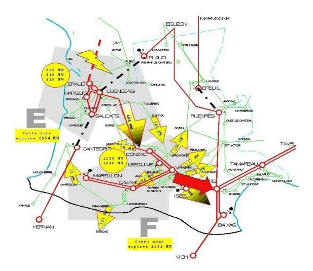
Figure 8-13: Initial Fault leading to the exceeding of the maximum transfer capacity
