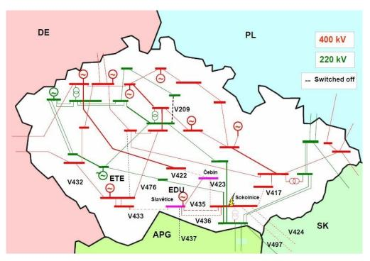
FIGURE 8-8: ON LINE SCHEME OF TRANSMISSION SYSTEM IN 14:51
