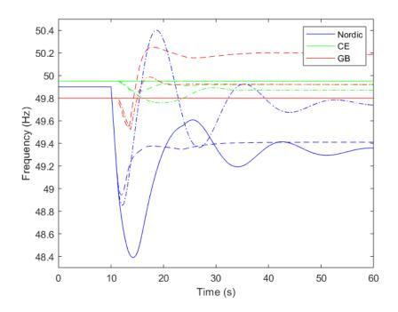
Figure 15: Power loss of 1.5 times the reference incident in the **Nordic system**, scenario 2030 low inertia (Solid curves: represent no support, - dash: proportional to frequency deviation, dash-dot: step support).
