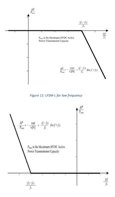
Figure 12: LFSM-U for over frequency
