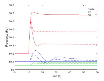
Figure 16: Demand loss of 1.5 times the reference incident **in the GB system**, scenario 2030 low inertia for over frequency support (Solid curves: represent no support, - dash: proportional to frequency deviation, dash-dot: step support)
