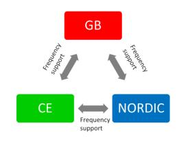
*Figure 9* : GB, CE and Nordic frequency control model connected by HVDC links
