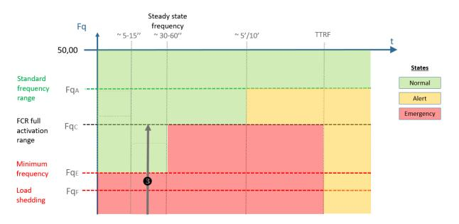
Figure 7: Frequency support relating to duration of the emergency state of requesting synchronous area
