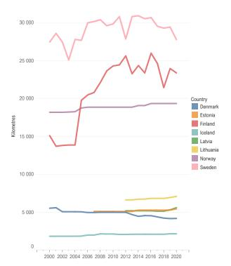
Figure E.6: Length of overhead lines (km) in the 100–420 kV grids at the end of each year. Estonia has data since 2007, and Latvia and Lithuania have data since 2012.
