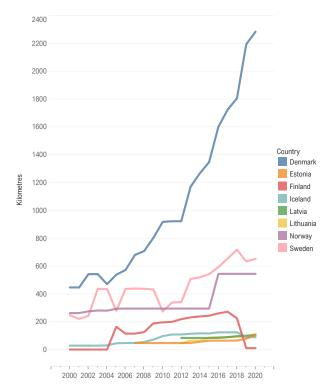
Figure E.5: Length of cables (km) in the 100–420 kV grids at the end of each year. Estonia has data since 2007, and Latvia and Lithuania have data since 2012.
