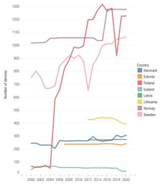
Figure E.8: Number of instrument transformers in the 100–420 kV grids at the end of each year. Estonia has data since 2007, and Latvia and Lithuania have data since 2012.
