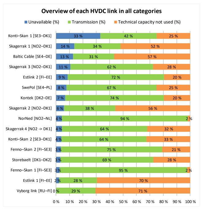
FIGURE C-1 ANNUAL OVERVIEW OF EACH HVDC LINK SORTED BY DESCENDING UNAVAILABLE TECHNICAL CAPACITY (Eu) IN 2015
