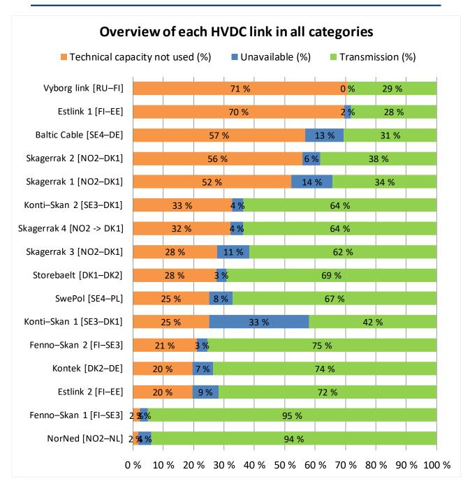
FIGURE C-3 ANNUAL OVERVIEW OF EACH HVDC LINK SORTED BY DESCENDING TECHNICAL CAPACITY NOT USED (ETCNU) IN 2015
