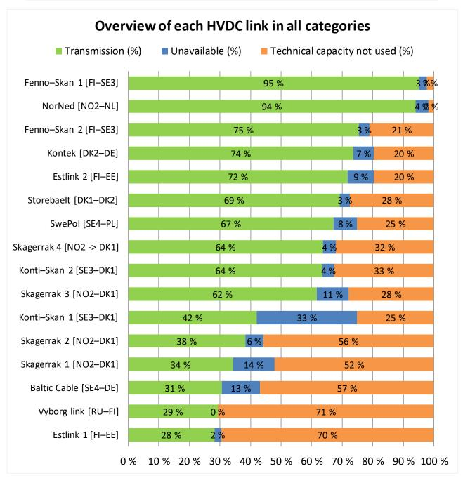
FIGURE C-2 ANNUAL OVERVIEW OF EACH HVDC LINK SORTED BY DESCENDING TRANSMISSION ( $E_{T}$ ) IN 2015
