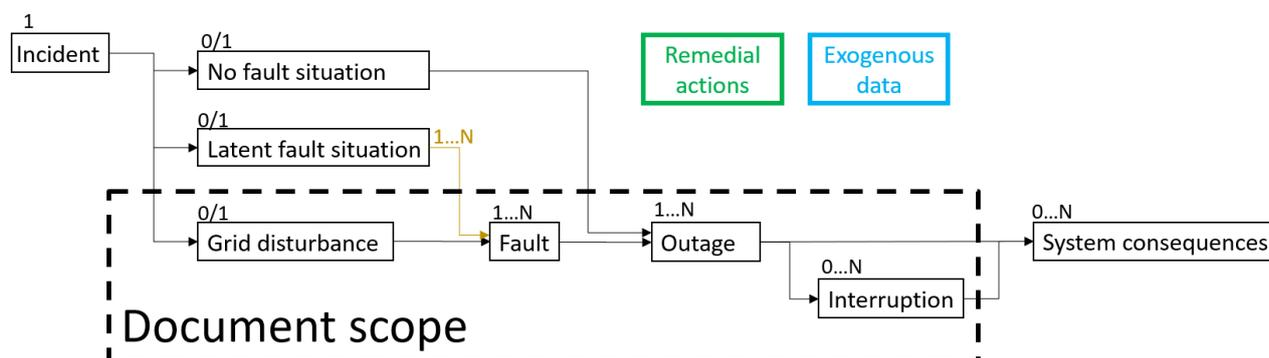
Figure 5.1 The situation after an incident is called a ‘no fault situation’, a ‘latent fault situation’ or a grid disturbance based on the involvement of faults. A grid disturbance is caused by faults and a fault can result in several outages. Outages can also result in none, one or several interruptions which may affect end-users and result in energy not supplied (ENS).
