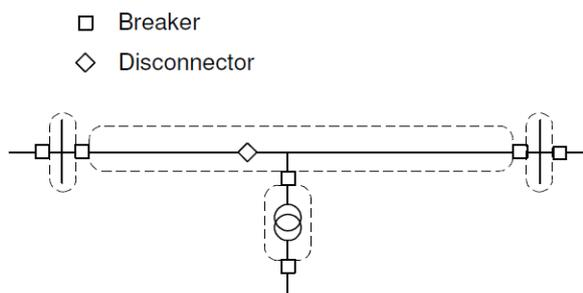
Figure 4.11 A system unit is delimited by circuit breakers as indicated by the dotted lines. Disconnectors do not delimit system units. This system unit must be defined as being of the line type.
