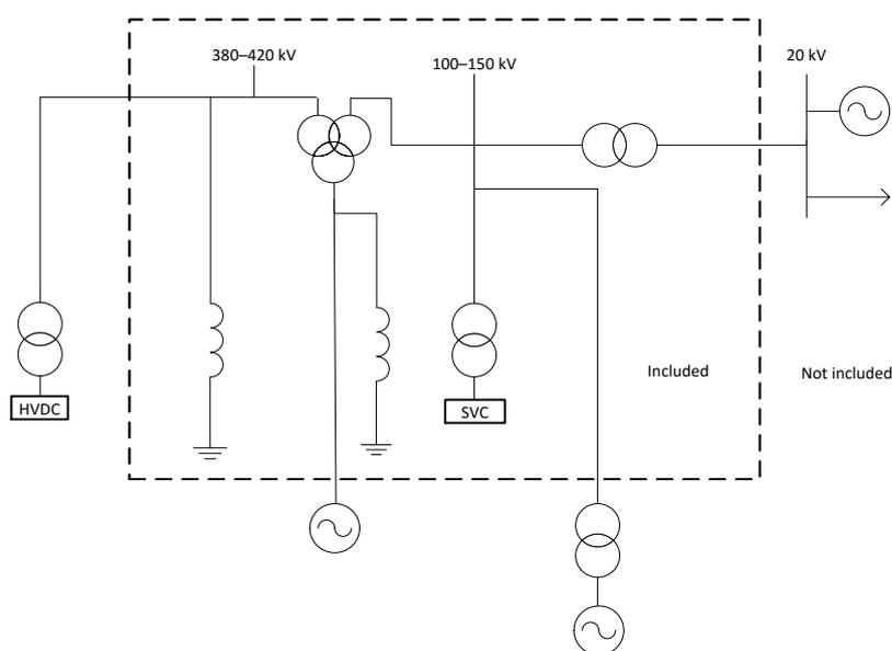
Figure .42.1 The dashed-line rectangle shows the types of components which are included in the classification
