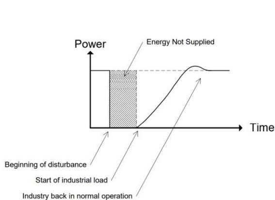
Figure 4.4 Grid disturbance with end-user interruption for industrial load. The interruption ends when voltage is supplied at the delivery point.
