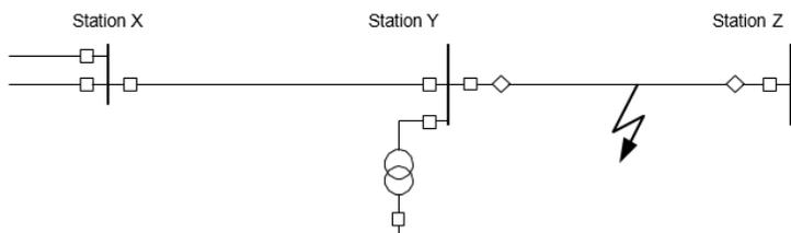
Figure 0.8 Line fault and fault in the high-speed automatic reclosing equipment.
