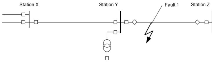
Figure 0.14 Earth fault in a compensated network with latent relay fault.
