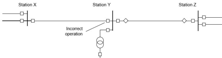
Figure 0.3 Incorrect circuit breaker operation.
