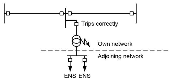
Figure 4.9 ENS must be recorded when the transformer is affected by a fault that causes an outage.
