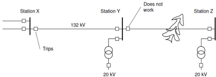
Figure 0.15 Fault on a radial feeder line with circuit breaker failing to trip.
