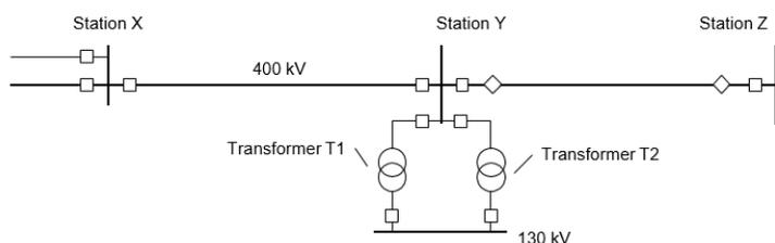
Figure 0.19 Outage of parallel power transformers due to tap changer fault and overload.
