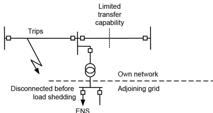
Figure 4.6 ENS due to transmission restrictions. A delivery point is disconnected because there is not enough transmission capacity.
