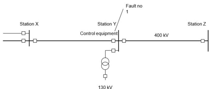
Figure 0.11 Unsuccessful power transformer energisation due to sensitive relay settings.
