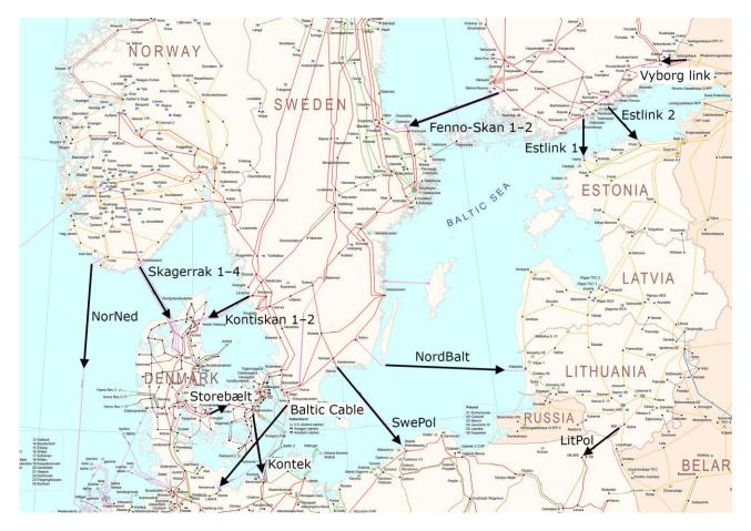
FIGURE 2.1 PART OF THE NORDIC GRID MAP SHOWING THE HVDC LINKS [1]. THE ARROWS INDICATES THE DIRECTION OF EXPORT USED IN THIS REPORT.
