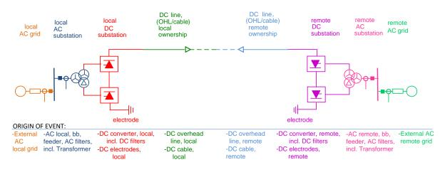
FIGURE A-1 A SCHEMATIC PRESENTATION OF A HVDC LINK WITH LINE COMMUTATED CONVERTERS (LCC)
