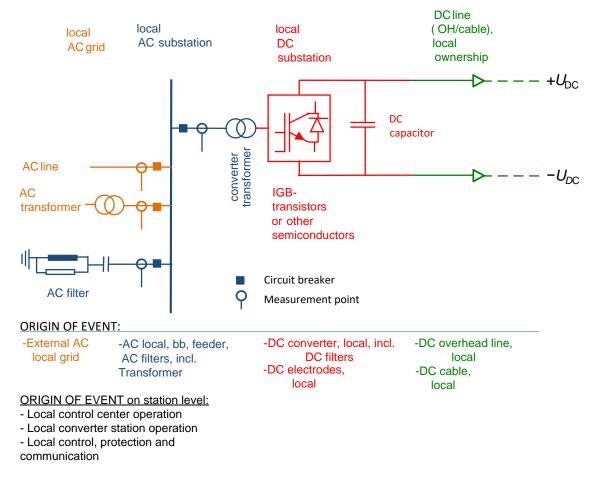
FIGURE A-4 A CONVERTER STATION OF A VOLTAGE SOURCE CONVERTER HVDC LINK WITH THE CONNECTION TO THE AC GRID
