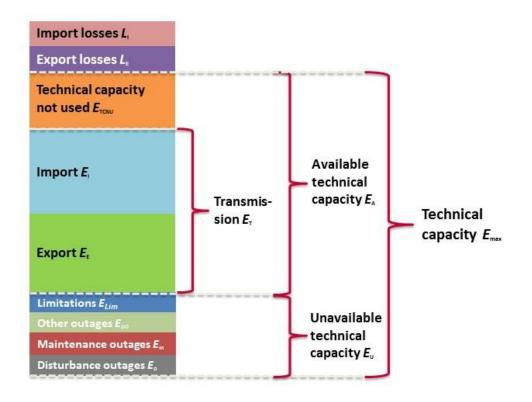
FIGURE 4.1 THE AVAILABILITY AND UTILISATION CATEGORIES USED IN THE HVDC STATISTICS. THE DEFINITIONS AND CALCULATIONS ARE EX-PLAINED IN CHAPTER 4. EVERY VALUE IS AN ENERGY VALUE AND REPRESENTS A PART OF THE AVAILABLE OR UNAVAILABLE TECHNICAL CAPACITY. THE NINE CATEGORIES OF THE COLUMN TO THE LEFT ARE INTERNALLY EXCLUSIVE AND THEIR SUM AMOUNTS TO THE TOTAL TECHNICAL CAPACITY.
