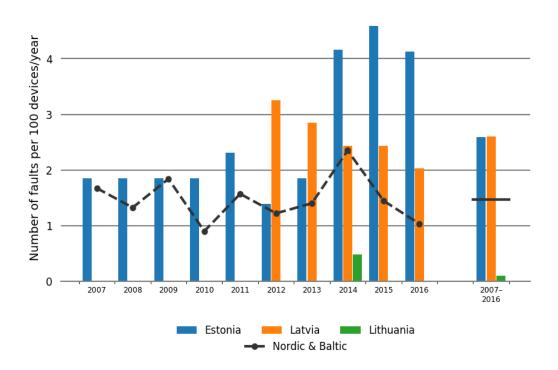
Figure 5.5.5 Annual distribution of faults for 100–150 kV power transformers and the average for Estonia during 2007–2016 and for Latvia and Lithuania during 2012–2016
