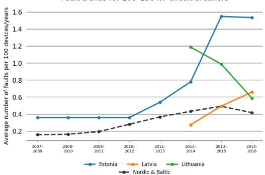
Fault trends for 100-150 kV circuit breakers
