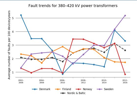
Figure 5.5.6 Fault trends as five-year averages for 380–420 kV power transformers in Nordic countries
