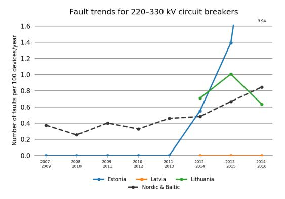
Figure 5.7.3 Fault trends as three-year averages for circuit breakers at the voltage level 220–330 kV in each Baltic country. Estonia has reported data since 2007 and Latvia and Lithuania have reported data since 2012.
