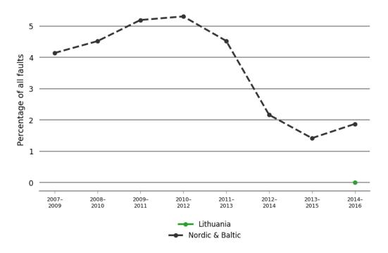
Figure 6.6.13 Fault trends as three-year averages for 380–420 kV operation and maintenance for Lithuania. Lithuania has reported data since 2012.
