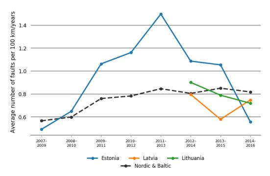
Fault trends for 220-330 kV overhead lines
