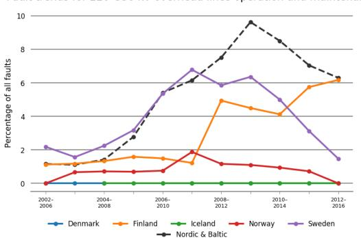
Fault trends for 220–330 kV overhead lines operation and maintenance
