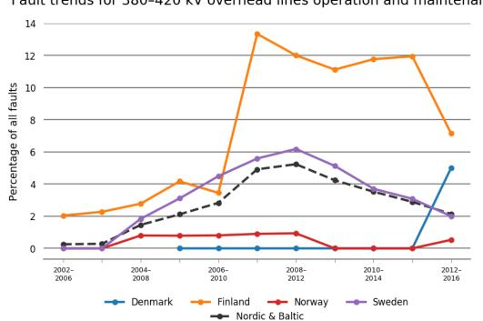
Fault trends for 380–420 kV overhead lines operation and maintenance
