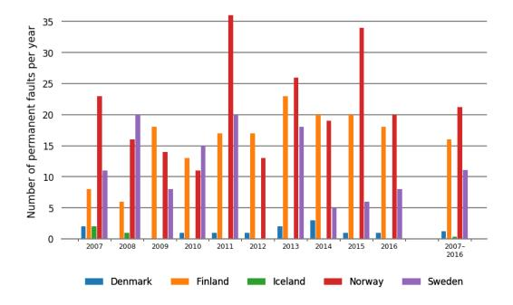
Figure 5.3.8 Annual distribution of permanent faults for 100–150 kV overhead lines during the period 2007–2016 and the average for 2007–2016 in each Nordic country
