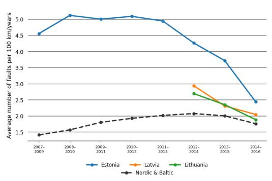
Fault trends for 100-150 kV overhead lines
