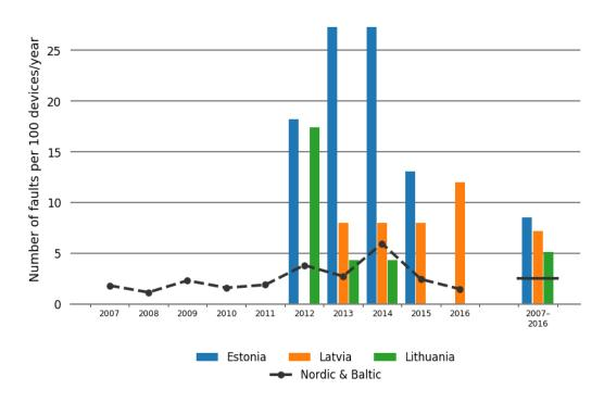
Figure 5.5.3 Annual distribution of faults for 220–330 kV power transformers and the average for Estonia during 2007–2016 and for Latvia and Lithuania during 2012–2016
