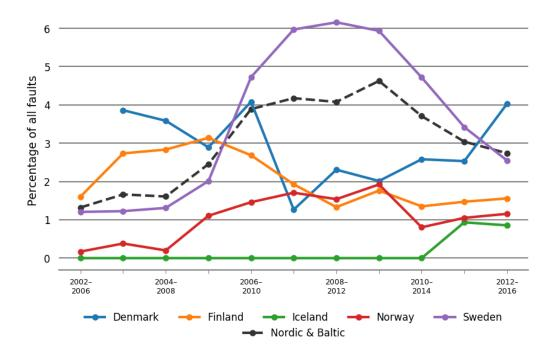
Fault trends for 100–150 kV overhead lines operation and maintenance
