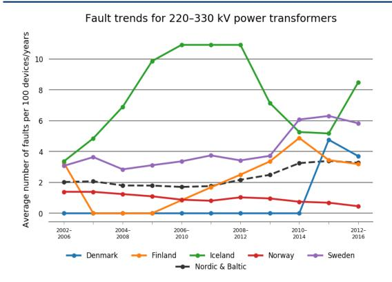
Figure 5.5.7 Fault trends as five-year averages for 220–330 kV power transformers in each Nordic country
