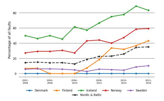
Fault trends for 220–330 kV overhead lines other environmental causes
