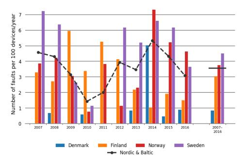
Figure 5.8.1 Annual distribution of 380-420 kV control equipment faults and the average for the period 2007-2016
