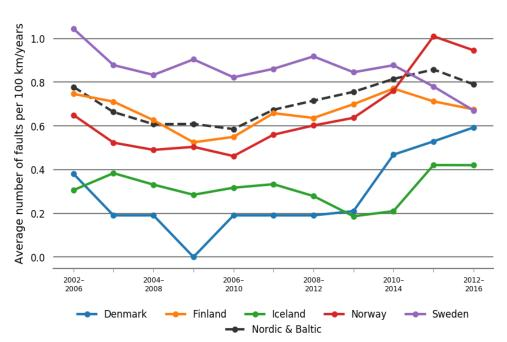
Fault trends for 220–330 kV overhead lines
