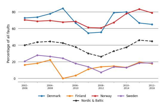
Fault trends for 380-420 kV overhead lines other environmental causes
