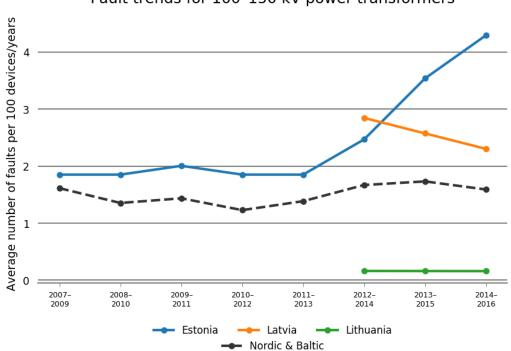
Fault trends for 100-150 kV power transformers
