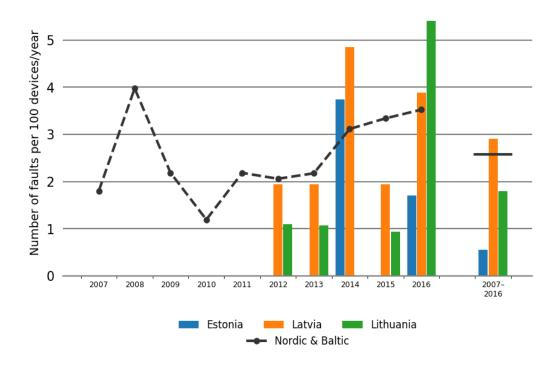
Figure 5.8.3 Annual distribution of 220-330 kV control equipment faults and the average for Estonia during 2007-2016 and for Latvia and Lithuania during 2012–2016
