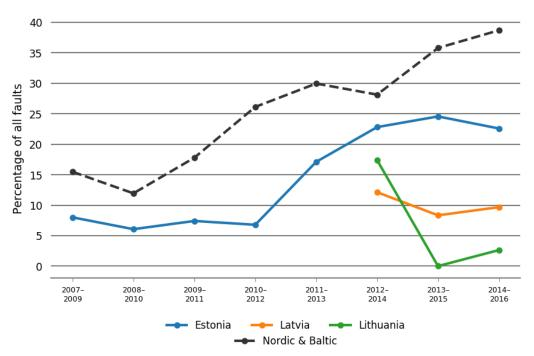
Fault trends for 220–330 kV overhead lines other environmental causes
