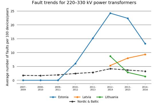
Figure 5.5.8 Fault trends as three-year averages for 220–330 kV power transformers in each Baltic country. Estonia has reported data since 2007 and Latvia and Lithuania have reported data since 2012.
