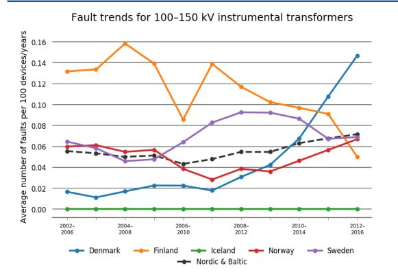
Figure 5.6.4 Fault trends as five-year averages for instrument transformers at the voltage level 100–150 kV in each Nordic country
