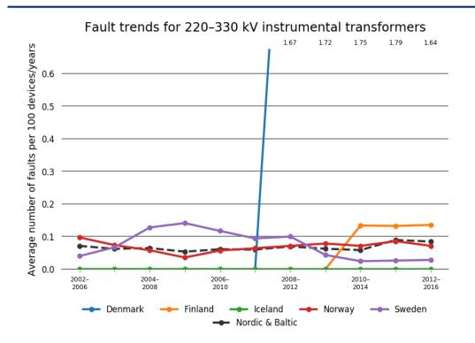
Figure 5.6.2 Fault trends as five-year averages for instrument transformers at the voltage level 220–330 kV in each Nordic country
