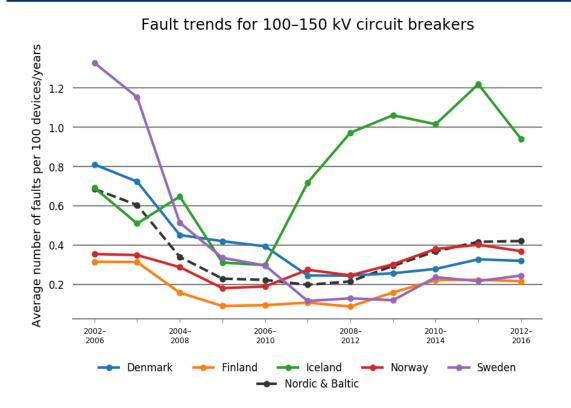
Figure 5.7.4 Fault trends as five-year averages for circuit breakers at the voltage level 100–150 kV in each Nordic country
