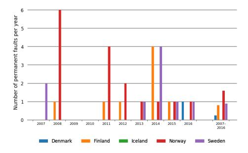
Figure 5.3.1 Annual distribution of faults for 380–420 kV overhead lines during the period 2007–2016 and the average for 2007–2016 in Nordic countries
