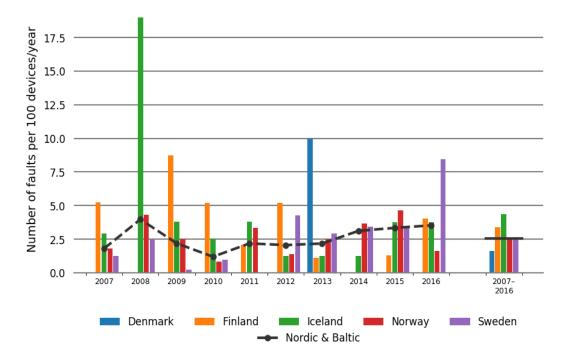
Figure 5.8.2 Annual distribution of 220-330 kV control equipment faults and the average for the period 2007-2016 for each Nordic country
