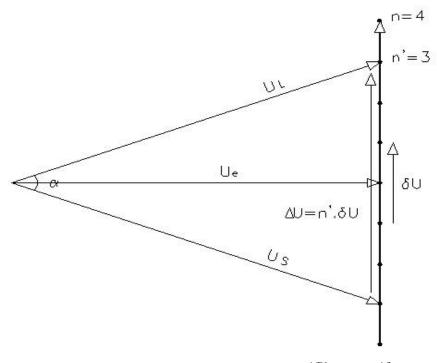
While in the basic semantic model (figure 2),  $\alpha = 2 \arctan \frac{n' \delta U}{2U_e} = 2 \arctan \frac{n' \delta u}{2}$  and  $\rho = 1$ . Ue is the central voltage (kV) Figure 7. Symmetrical (Type = SYMM)
