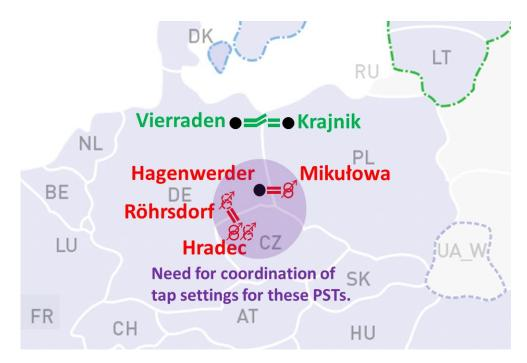
Figure 21: Existing (solid line) and planned / under construction (dotted line) PSTs in the region.
