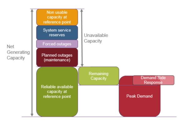
Figure 4: Upward adequacy methodology.
