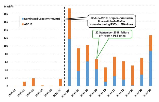
Figure 22: Average monthly import capacity on synchronous profile with DE+CZ+SK before and after reconfiguration on PL-DE border.
