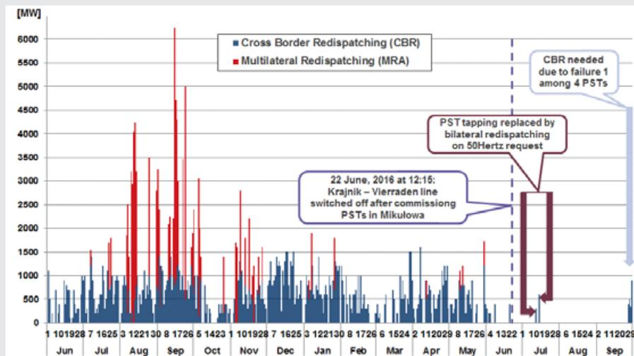
Figure 2: Maximum daily volume of CBR and / or MRA necessary to keep 50Hertz / PSE profile in N-1 secure state.
