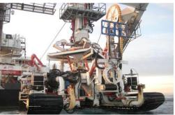
Trencher used by Eirgrid for burying the cable of the East-West Interconnector
