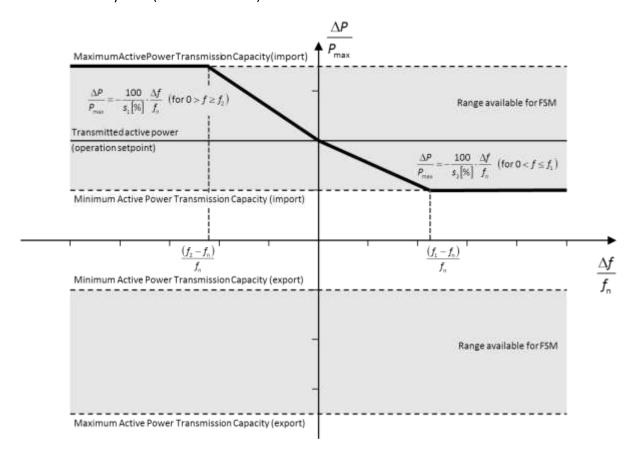
Figure 1: Active Power Frequency Response capability of a HVDC System in FSM illustrating the case of zero deadband and insensitivity with a positive Active Power Setpoint (import mode).  $\Delta P$  is the change in Active Power output from the HVDC System.  $f_n$  is the target Frequency in the AC Network where the FSM service is provided and  $\Delta f$  is the Frequency deviation in the AC Network where the FSM service is provided.
