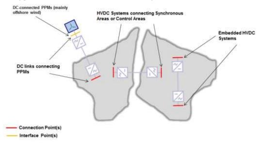
*Example 1: Illustration of the Significant Grid Users considered in the NC HVDC and the Connection Points and Interface Pont(s) at which the requirements apply.*
