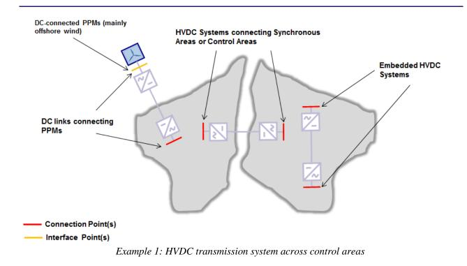
An HVDC system with AC/DC terminals across multiple synchronous areas or control areas, has a crossborder impact since a fault in the HVDC system causes a change of flows between control areas. Therefore these schemes are deemed to be Significant Grid Users.
