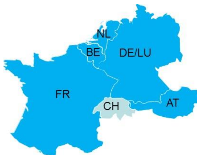
Figure A3: Bidding zones of the CCR CWE (DE/LU - AT bidding zone border is not part of this CCR)
