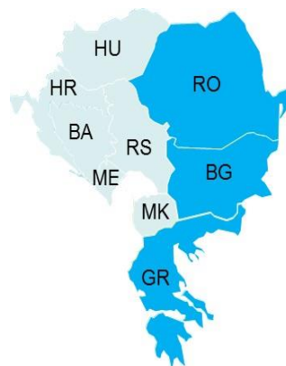
Figure A11: Bidding zones of the CCR SEE (HU-RO and HU-HR bidding zone borders are not part of this CCR)
