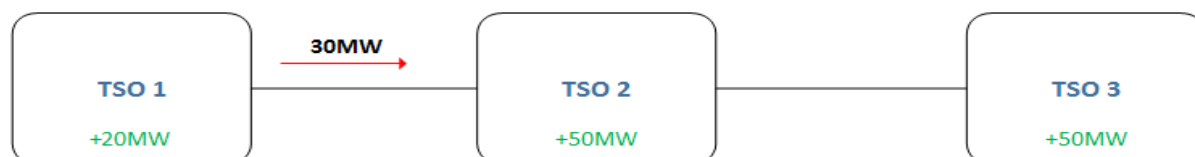
Figure 22 - Topology of the example illustrating interconnector controllability
