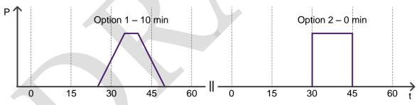
Figure 14 : Illustration of the two options for the ramp duration of the cross border echange
