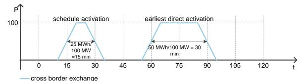
Figure 7: illustration of the equivalent delivery period for a schedule activation and the earliest direct activation of the merged mFRR product
