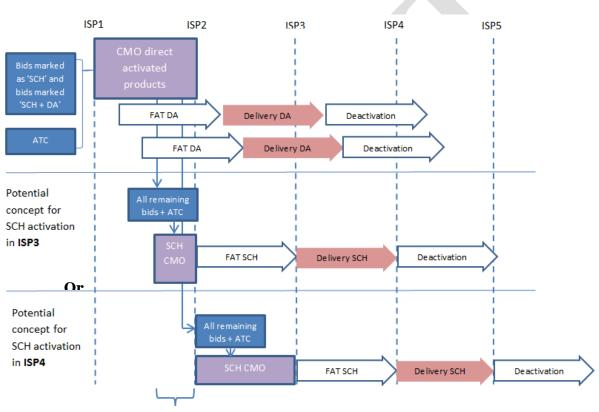
Note, period of time needed for SCH process to run algorithm and optimise (including netting where possible) all TSO requests to allow FAT over ISP2 and delivery in ISP3. Potential issue with simultaneous SCH process where DA activations still occurring from same CMO
