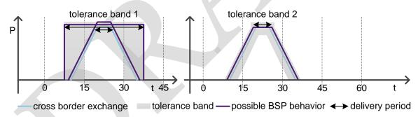
Figure 6: illustration of different tolerance bands and their influence on delivery period in the case of a schedule activation with a fixed shape of the cross border exchange of the merged mFRR product. Since the tolerance band can be defined by each TSO individually, it is not possible to define a global minimum and maximum delivery period.
