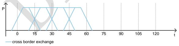
Figure 16: illustration of the shape of the cross border exchange for the RR project used in the TERRE project
