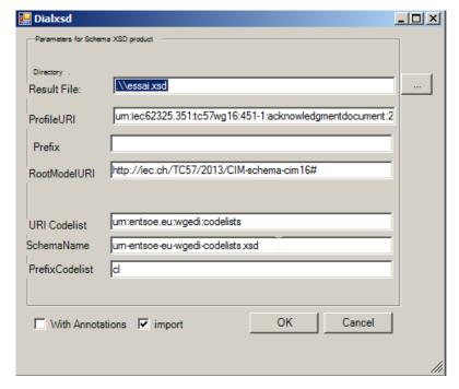
Figure 41 - CIMSyntaxgen dialog box to generate a XSD (import option)
