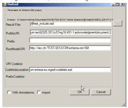
Figure 42 – CIMSyntaxgen dialog box to generate a XSD (no import option)
