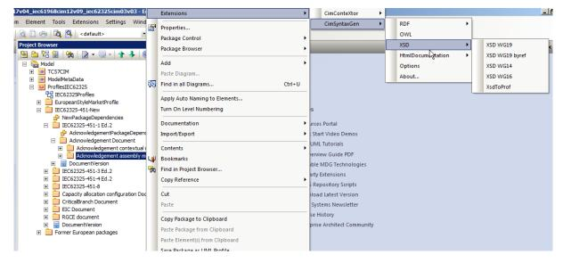
Figure 40 - Running CIMSyntaxgen to generate a XSD
