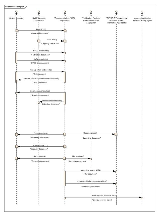
Figure 2: The replacement reserve process sequence diagram
