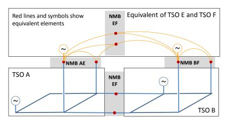
Figure 5 Equivalent from Fully Reduced TSO E and TSO F Networks
