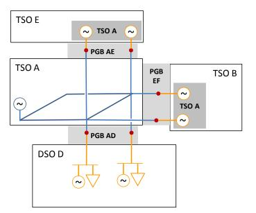
Figure 4 Example where TSO A has replaced TSO B and TSO E with Network Edges
