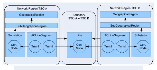
Figure 3 Detailed CIM data diagram for the tie line between tso a and tso b
